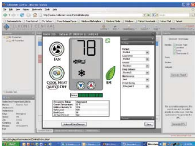
HVAC room settings can be easily changed with the touch of a few buttons on the virtual thermostat.
